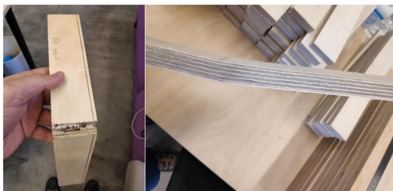
Figure 4. Test pieces after bending tests, showing brittle failure in black alder ( left ), and ductile failure in aspen ( right ) plywood.
