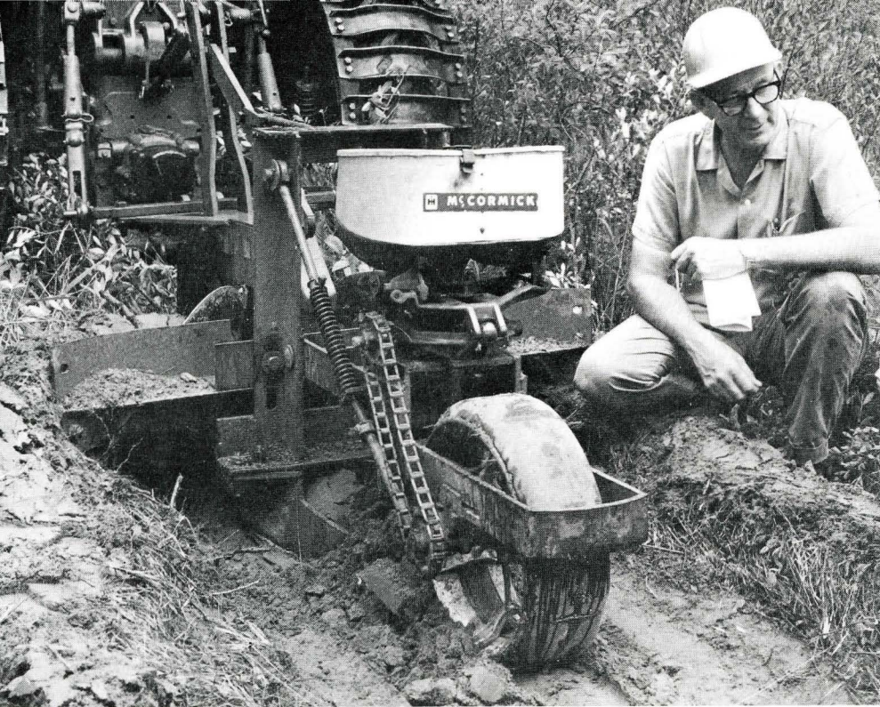
A furrow seeder that operates behind a conventional fireplow. Adjustable hillers elevate a ridged bed in the center of the furrow to prevent washing and flooding of the seeds.
