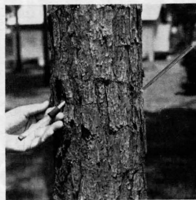
To measure the viscosity of gum researchers first collected it in a viscosity tube (in hand) attached to the tree. At right is a capillary tube inserted to measure pressure of exudation, another delicate experiment.
