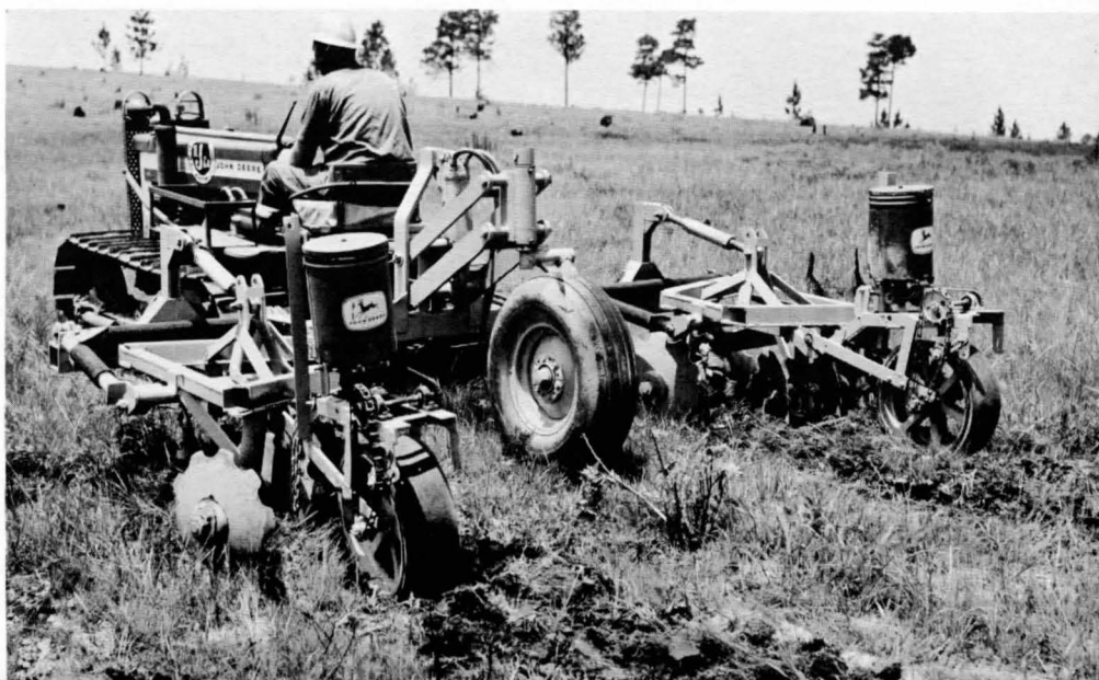
Disk seeders prepare a narrow bed and sow seed in a single pass. Two-row models have been developed; the one shown here makes a flat bed.
