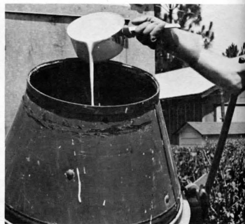
To 50 pounds of seed, add 1.2 gallons of the repellent as mixer is turning. Tumble for about 2 minutes.
