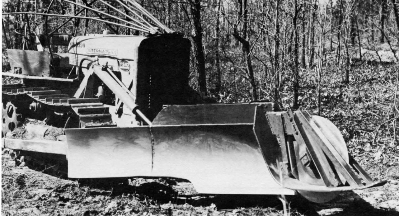
This front-end model has the seed hopper just behind the point of the V-blade. It operates effectively in dense brush.
