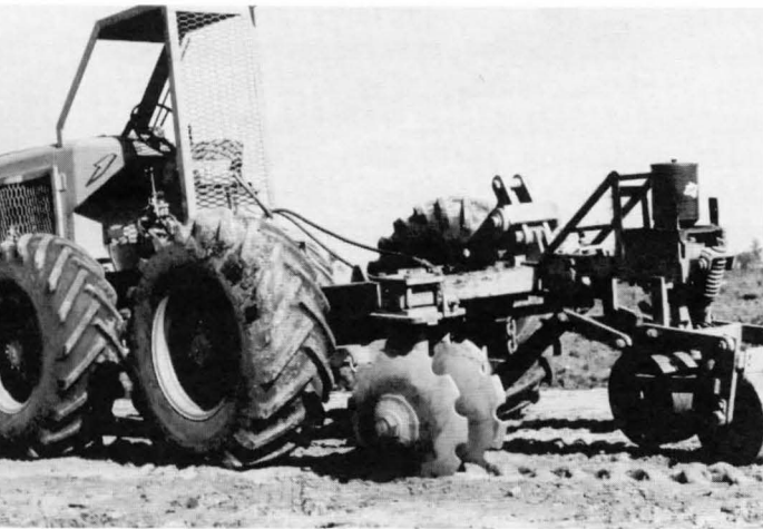
This heavy-duty seeder elevates a bed 12 inches high and 6 feet wide.
