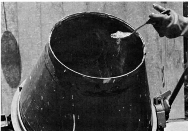
Add aluminum powder and tumble for another minute.
