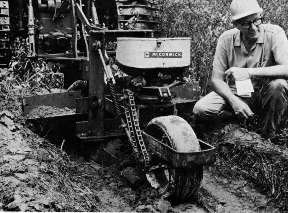
This model of the H-C Furrow Seeder operates behind a conventional fire-plow. Adjustable hillers elevate a ridge in the center of the furrow to prevent washing or flooding of the seed.
