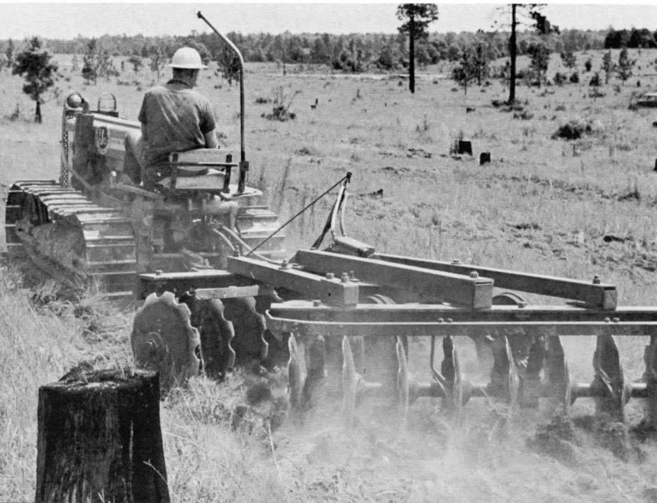
On rolling uplands, a light offset disk prepares satisfactory seedbeds.
