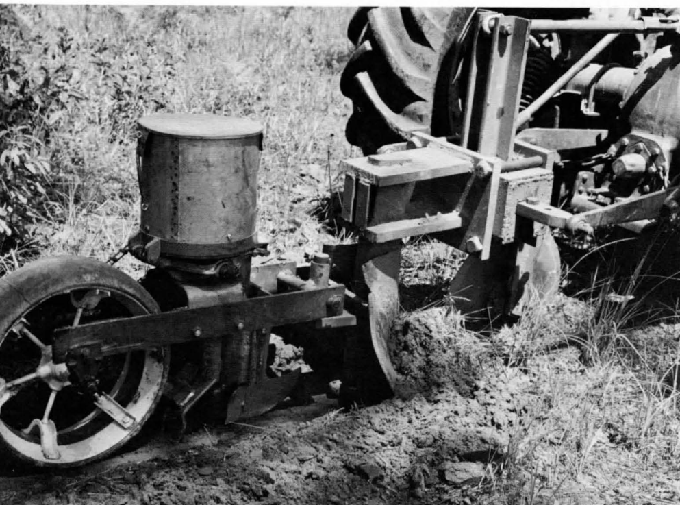
Light, compact seeders are designed for sandy soils. Most models drop seeds in a narrow furrow and cover them lightly.
