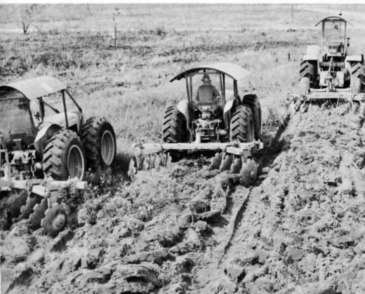
On poorly drained flatwoods soils, disked seedbeds are elevated to improve seedling growth.
