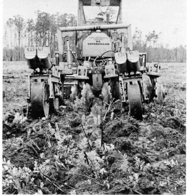
Two-row seeders are also available for sites requiring elevated beds.
