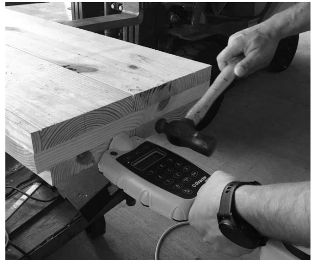
Figure 2—Longitudinal vibration evaluation of a three-ply CLT panel using a Hitman HM 200 tool.
