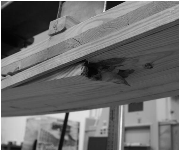
Figure 7—Static bending failure due to presence of knot.
