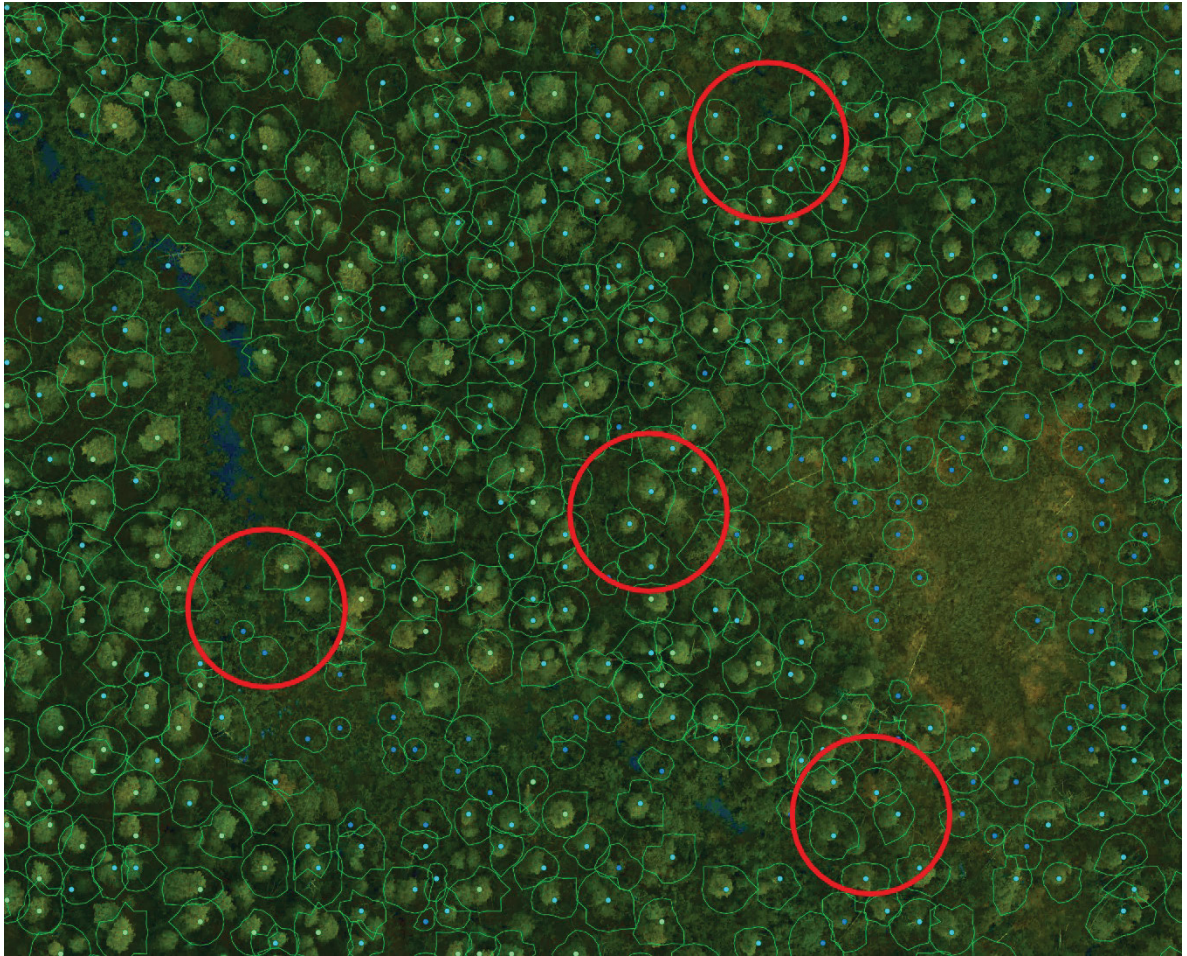
Figure 2—Example of LiDAR-based individual tree detection and measurement and high-resolution airborne orthorectification on a plot in interior Alaska. Red circles indicate subplots, green polygons represent tree crown segments, and blue dots are predicted stem locations (lighter blue represents higher crown heights).
