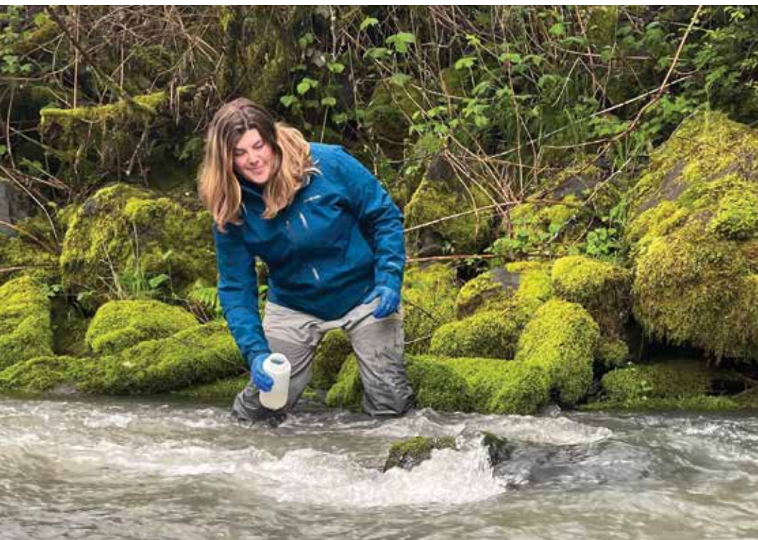
Brooke Penaluna, a research fisheries biologist with the Pacific Northwest Research Station, collects a water sample from Oak Creek in western Oregon. Environmental DNA is extracted from samples and analyzed in a lab to determine the species that live in and around the stream. Photo courtesy of Ivan Arismendi.
