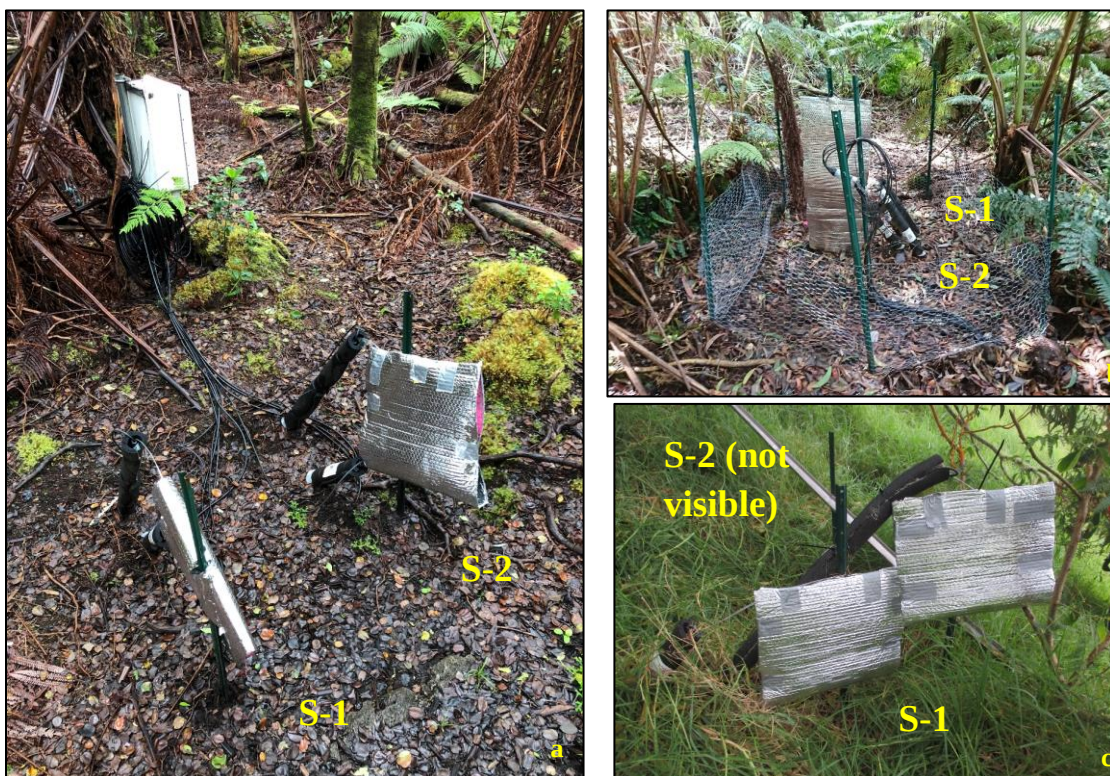
Figure 8. Soil-moisture measurement locations at (a) Nāhuku, Hawai'i (photo from Joseph Kennedy), (b) Laupāhoehoe, Hawai'i (photo from Han Tseng), (c) Nakula, Maui (photo from Alan Mair). S-1 and S-2 indicate soil moisture sensor locations.
