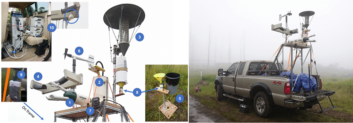
Figure 3. Instrumentation: (1) Phase Doppler Interferometer (Artium Technologies, Inc.), (2) Cloud Droplet Probe (Droplet Measurement Technologies, Inc.), (3) Juvik fog gauge, (4) visibility sensor, (5) rain gauge, (6) wind speed and direction monitor, (7) digital camera, (8) water isotope sampler, (9) aerosol spectrometer, (10) UAV sensor.
