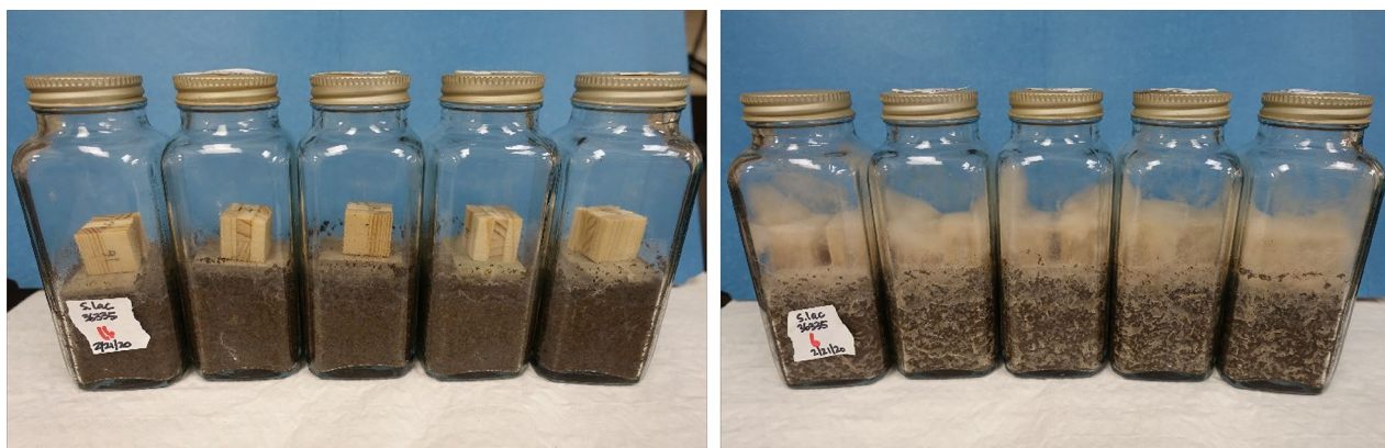
Fig. 14 Decay tests (AWPA E10–16) showing no visible fungal growth on borate-treated CLT blocks exposed to S. lacrymans for 12 weeks (left) and fungal growth on untreated CLT blocks exposed to S. lacrymans for 12 weeks (right)
