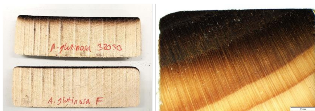
Figure 6. Transition zones of Alnus glutinosa contact charred at 320 °C (up) and flame charred (bottom), microscope image of transverse surface of spruce ( P. abies ) contact charred at 300 °C (bar 2 mm).
