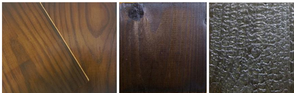
Figure 5. From left: Surfaces formed by compressive contact heating of pine at 260 °C, contact heating of spruce at 320 °C, gas flame charring of spruce (M. Kymäläinen).
