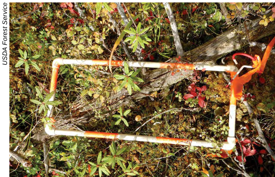
Figure 38—A Daubenmire microquad frame used to quantify ground layer composition and biomass. On each plot, ground layers were recorded at up to 32 locations along eight transects, when feasible (8 microquads and 2 transects per subplot).
