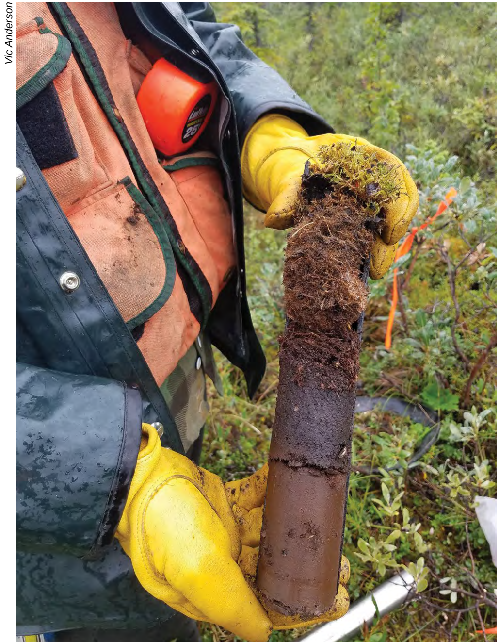
Figure 22—A Forest Inventory and Analysis crew member displays a soil core extracted from a plot in interior Alaska. Note the transition from green moss at the top of the core to decomposing organic material in the center and organic-rich mineral soil at the bottom of the core.
