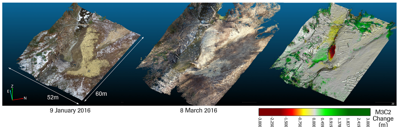
Fig. 13. Drone imagery of crib dam. (A) is RGB image and (B) is change detection within first month following removal of wooden crib dam.
