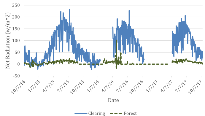
Fig. 8. Net radiation ( \text{w m}^{-2} (incoming short wave + long wave) – (outgoing short wave and long wave)) from a weather station in a clearing and a weather station in a nearby forest in the canopy interception study at the Priest River Experimental Forest.
