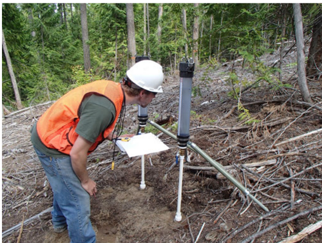
Fig. 4. Recording the change in infiltration with time with two constant head permeameters at the Montana biomass utilization study site. Note that the surface residue has been removed prior to setting up the permeameters.
