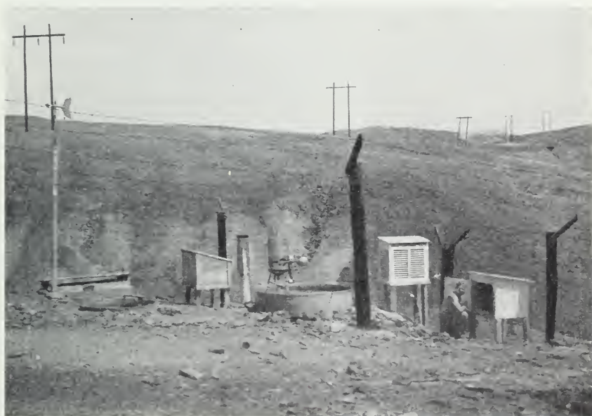
FIGURE 5.—One of the six meteorological stations. The instruments and shelters, reading from left to right, are: Wind vane, soil pit, evaporation pan, soil the mograph shelter, standard rain gage, recording rain gage, anemometer, class A Weather Bureau evaporation pan, minimum-maximum thermometer and hygrothermograph shelter, and microbarograph shelter. Other stations were similarly equipped.
