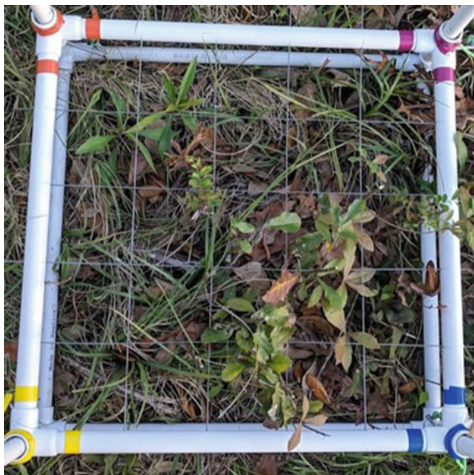
Fig. 2.9 Voxel sampling frame, vertical view showing the 10 \times 10 \times 10 cm sample voxel grid of a mixed shrub, herb, grass, and litter fuelbed (Photo by Susan Prichard)
