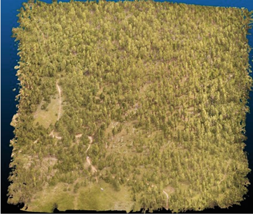
Fig. 2.3 Structure from motion point cloud generated for a mixed conifer site (roughly 500 m by 500 m in size) at the Lubrecht Experimental Forest, Montana
