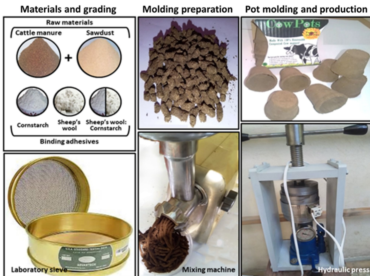
Fig. 1 Pot production. Materials and equipment used in this study
