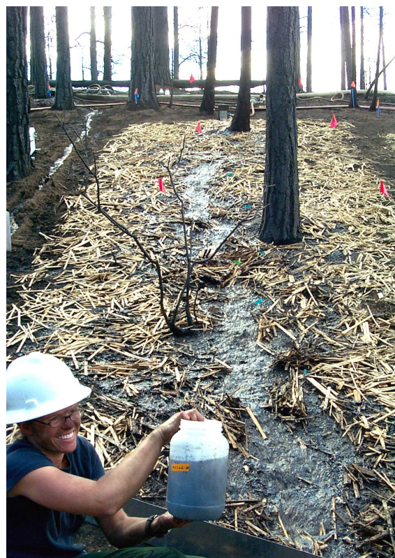
Collecting sediment-laden runoff from a hillslope plot with wood shreds after the 2002 Hayman Fire. USDA Forest Service photo by Pete Robichaud.
