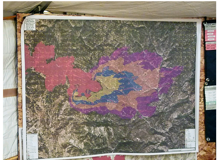
WindNinja winds in a fire progression simulation posted in a yurt in fire camp during the Pioneer Fire. (Courtesy photo by Jason Forthofer, Mechanical Engineer, Missoula Fire Sciences Laboratory).
