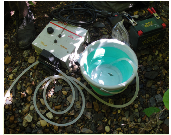
The basic equipment to collect an eDNA sample consists of a water pump, battery, and tubing to siphon water from the stream. The equipment fits in a small day pack that is easily carried by a hiker (Photo: USDA Forest Service, D. Isaak).
