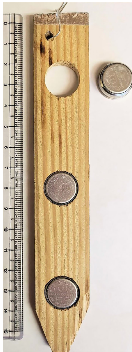
FIGURE 1 A complete iButton stake that will measure soil depths 5, 10, and 15 cm when installed with the top of the stake (picture left) 2 cm below the soil surface
