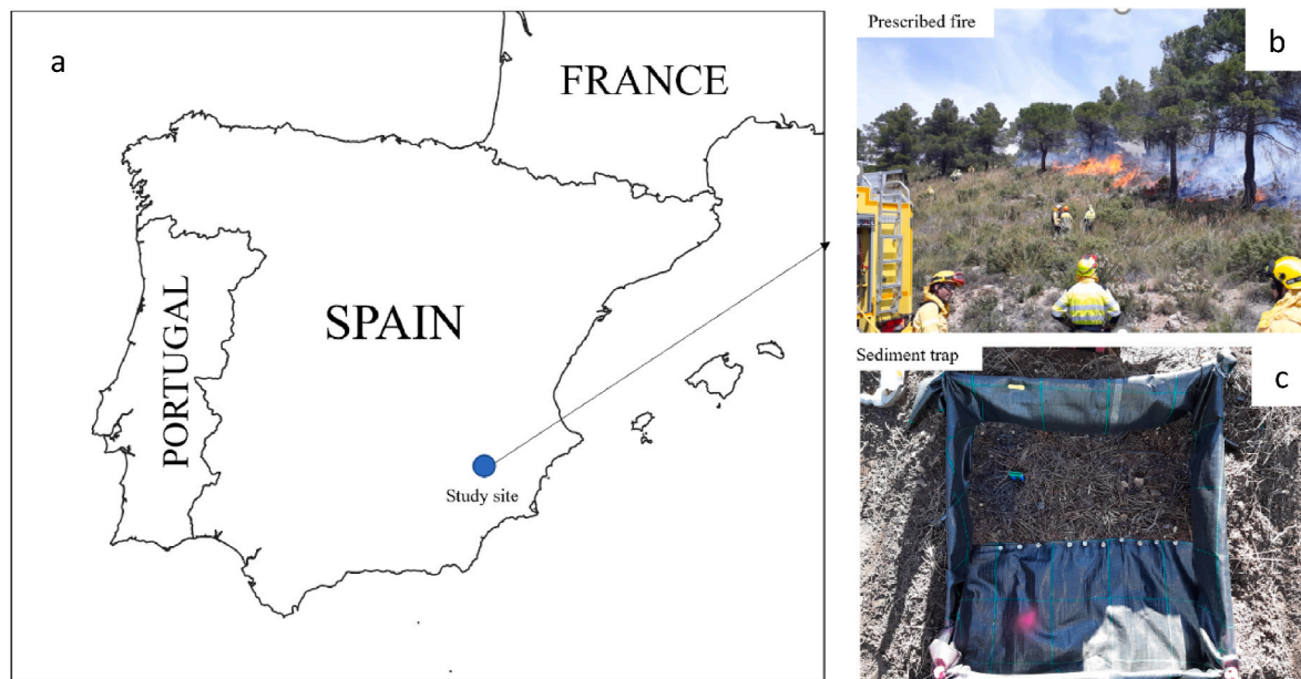
Fig. 1. Geographical location (a) of the study area (La Moraleja forest, Province of Albacete, Castilla La Mancha region, Spain); prescribed fire application (b); sediment trap to monitor rainsplash erosion (c).
