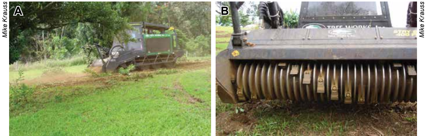
Figure 4.18—(A) Side view and (B) rear view of a masticator, which could be especially effective at treating Phellinus noxius -infected trees when these trees have already fallen to the ground.
