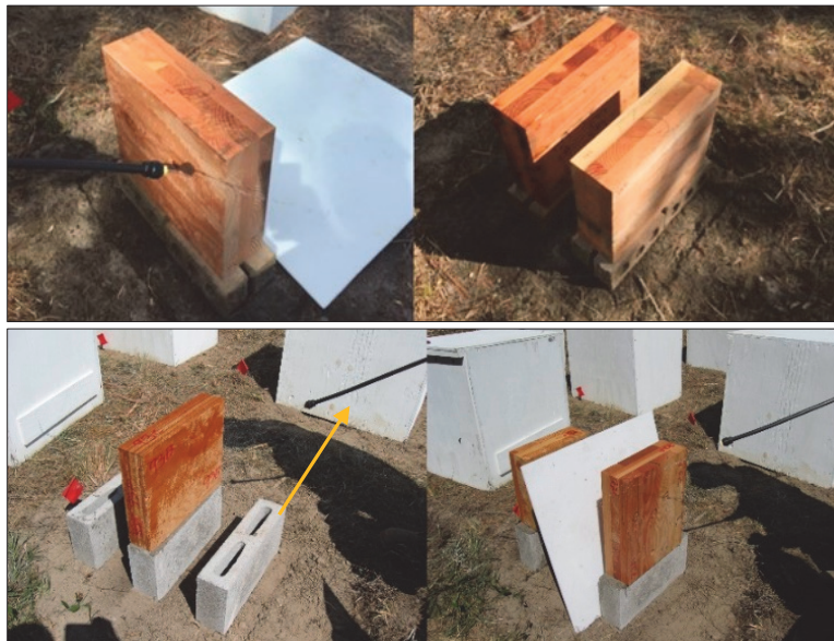
Figure 2. Photographs showing arrangement of ground bricks or cinder blocks and mass timber in subplots. Treatment with spray-on borate (23% DOT; arrow shows tip of spray nozzle) in the preventative and remedial treatments. Ground proximity test (top), above-ground test (bottom).
