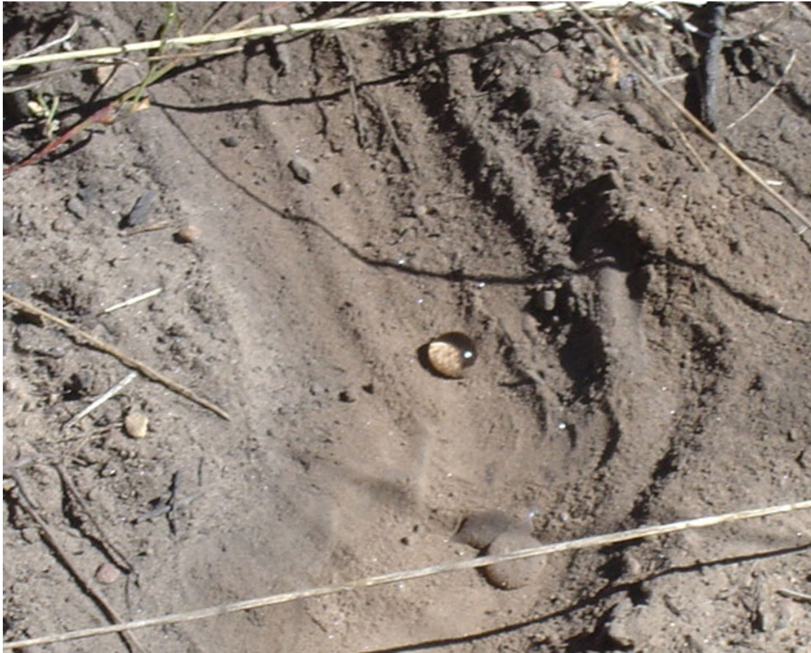
Figure 6. The time for a water droplet placed on a soil surface to penetrate into the surface is a measure of the level of water repellency of the soils at a sampling location. (Photo by Daniel G. Neary, USDA Forest Service)
