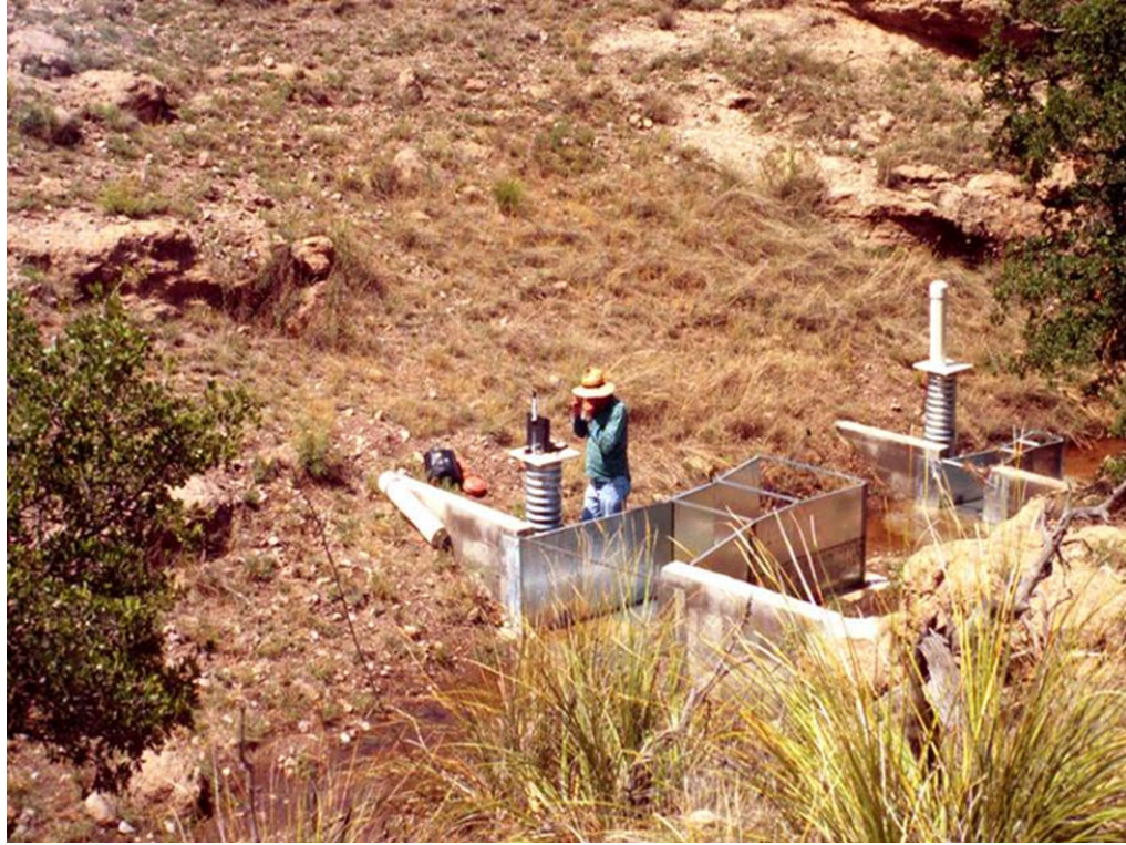
Figure 8. Two prefabricated Parshall flumes were installed on each of the Cascabel Watersheds to measure streamflow. A smaller flume measured low flows of water while the larger flume had a capacity to measure the infrequent larger flows. (Photo by Gerald Gottfried, USDA Forest Service).
