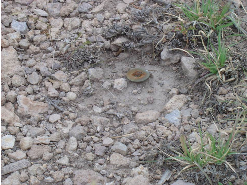
Figure 7. An erosion pin consisting of a metal nail with a washer welded to the top was inserted into the soil surface to measure soil erosion and deposition. The distance between the cap of the pin and the soil surface represented a measure of erosion while the amount of soil that accumulates on top of the cap was a measure of deposition. (Photo by Daniel G. Neary, USDA Forest Service).
