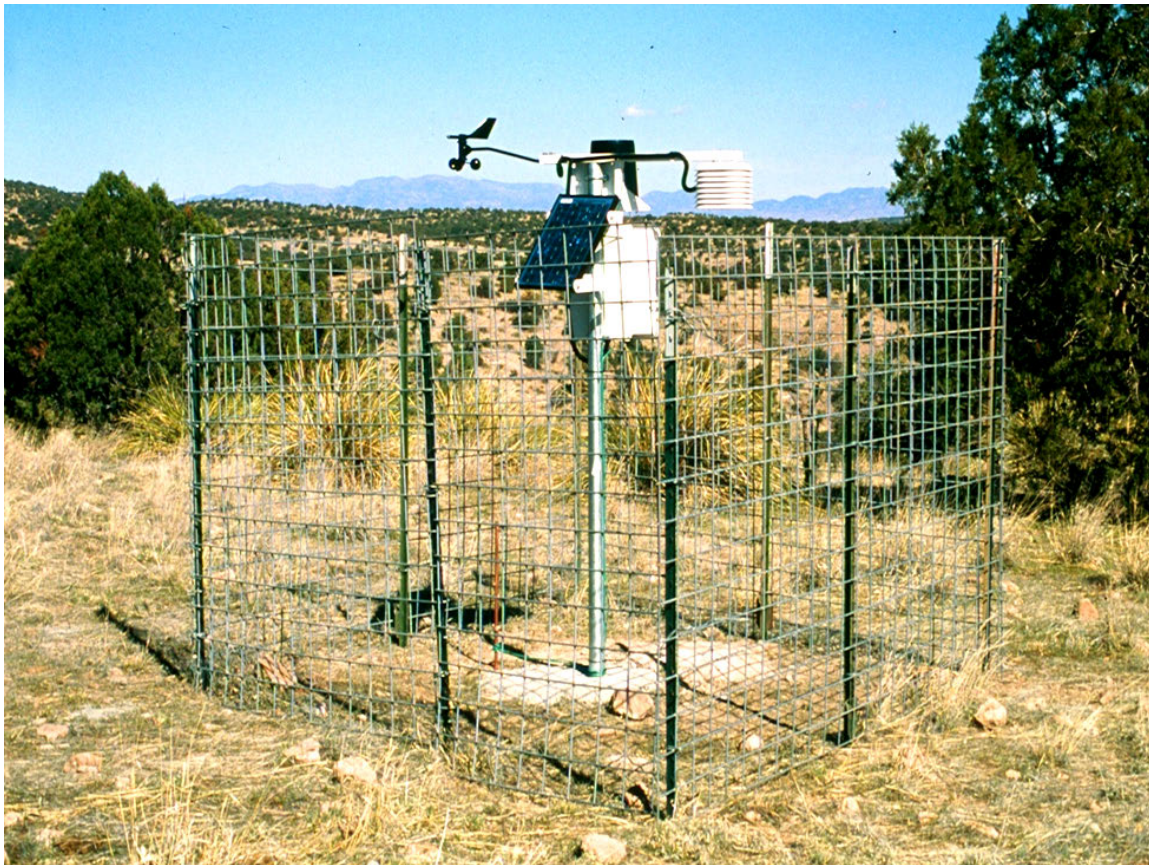
Figure 5. One of the two weather station installed on the Cascabel Watersheds to measure precipitation and other meteorological characteristics. (Photo by Gerald Gottfried, USDA Forest Service).
