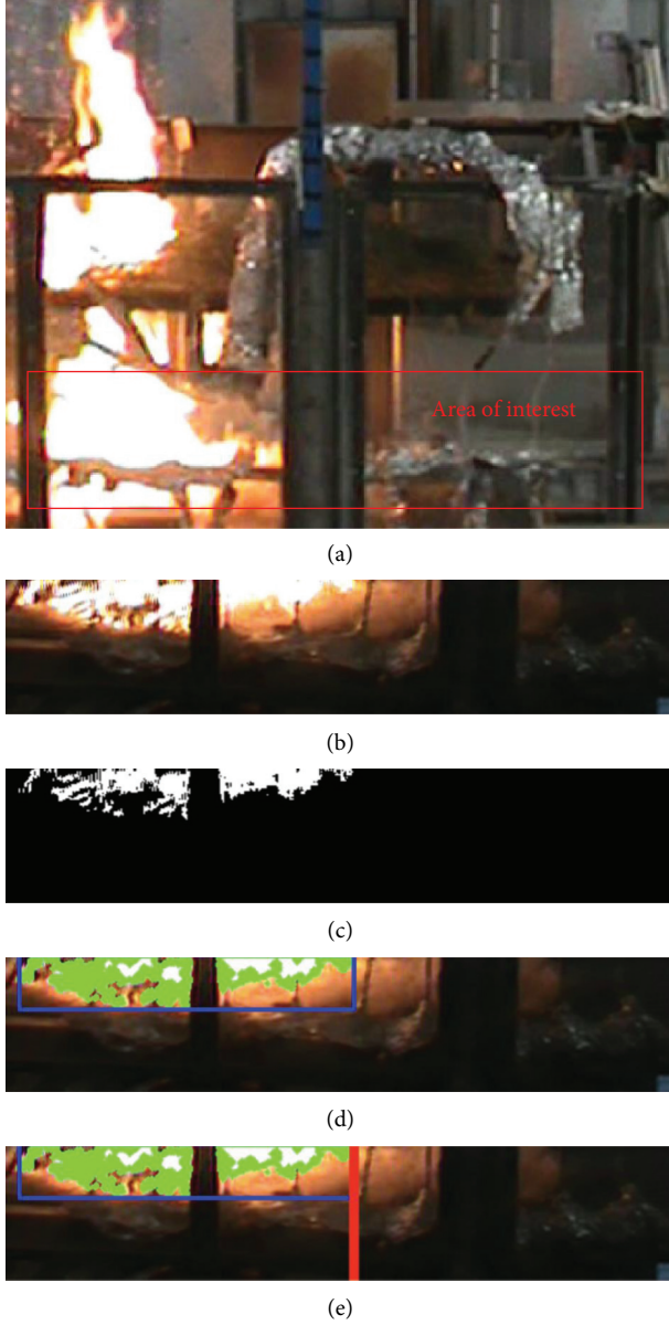
FIGURE 2: (a) Raw flame image. (b) Cropped flame region of interest. (c) Binary image. (d) Final bounding rectangle. (e) Identification of leading edge.
