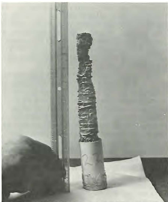
Figure 4.—Example of ice lens formation in pure kaolinite clay. The sample heaved 15 cm (200 percent) in 7 days. The closeup (right) shows little soil in the column, which indicates that the flow of heat to the freezing front was equal to the heat flow to the surface during most of the freezing period.
