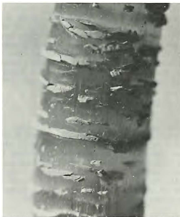
Figure 4.—Example of ice lens formation in pure kaolinite clay. The sample heaved 15 cm (200 percent) in 7 days. The closeup (right) shows little soil in the column, which indicates that the flow of heat to the freezing front was equal to the heat flow to the surface during most of the freezing period.
