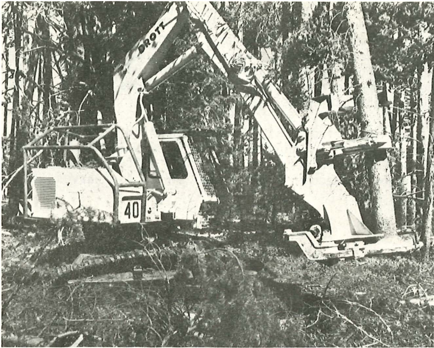
Figure 4.--A feller-buncher was employed on the Teton site to fell and bunch whole trees on the intensive utilization units.
