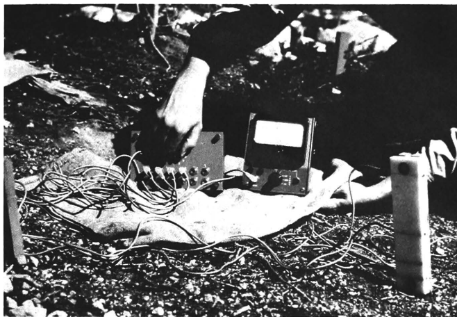
Figure 4.—Simultaneous air-temperature profiles were measured with unshielded thermistors at 2.5, 5.1, 10.2, and 20.3 cm above the surface using a tele-thermometer and switchbox.
