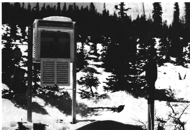
Figure 3.—Standard weather shelter installed on the north aspect showing hygrothermograph and max-min thermometer. Standard precipitation can is being weighed. Cup anemometer and generator in place (recorder not shown).
