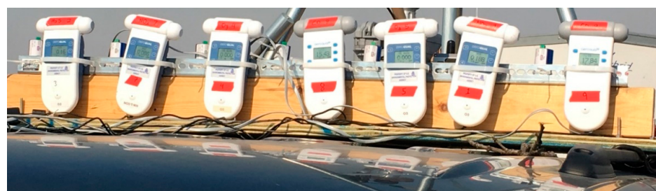
Figure 3. Close-up photograph of Aeroqual and Cairpol sensors mounted to the roof of the sampling vehicle.
