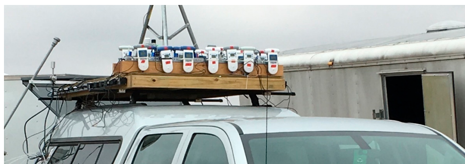
Figure 2. Photograph of Aeroqual and Cairpol sensors attached to the roof of the sampling vehicle from the November 2017 Konza and Tallgrass studies.
