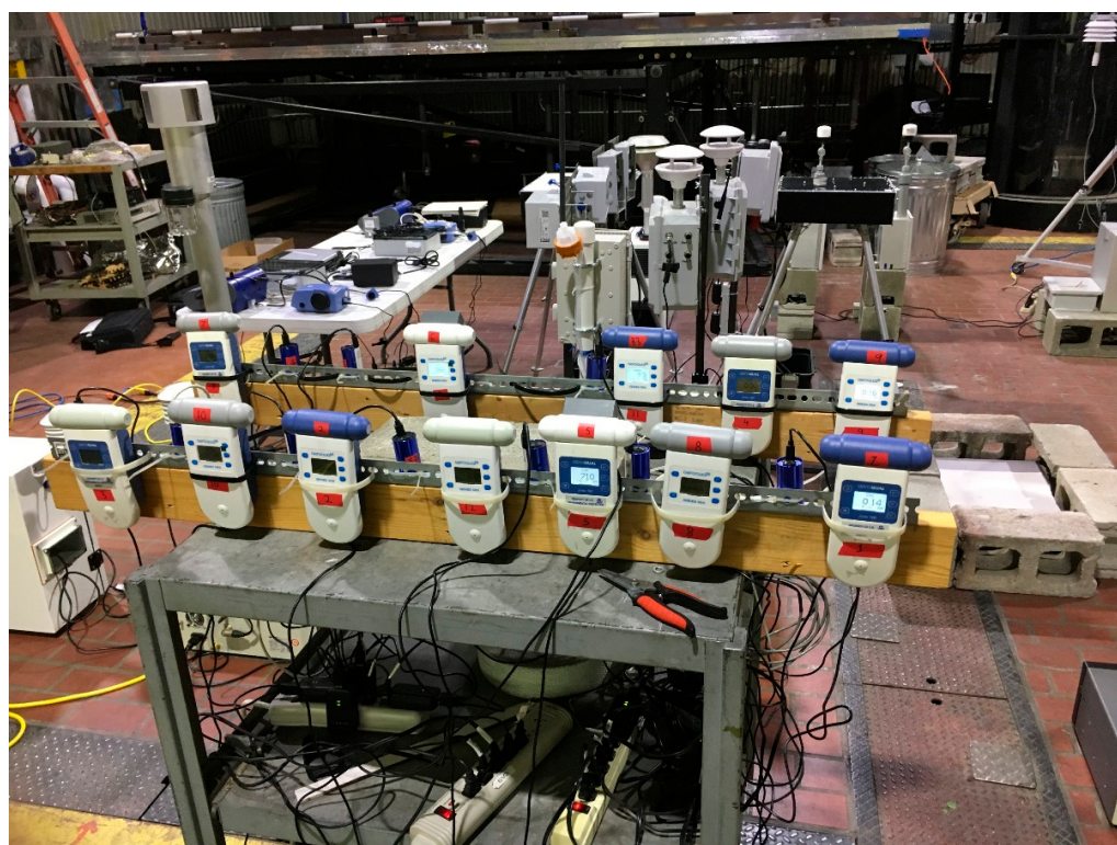
Figure 4. Photograph of Aeroqual and Cairpol sensors in the FSL.
