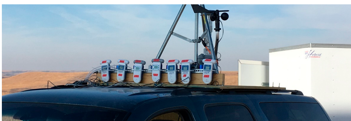
Figure 1. Photograph of Aeroqual and Cairpol sensors attached to the roof of the sampling vehicle from the March 2017 Konza study.
