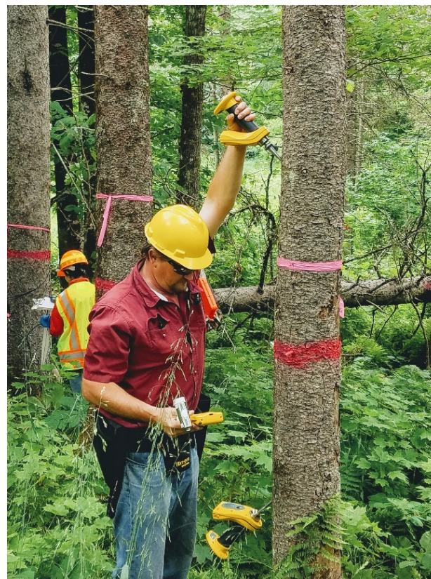
Figure 2. Longitudinal acoustic velocity measurements on white spruce trees using the Hitman ST300.
