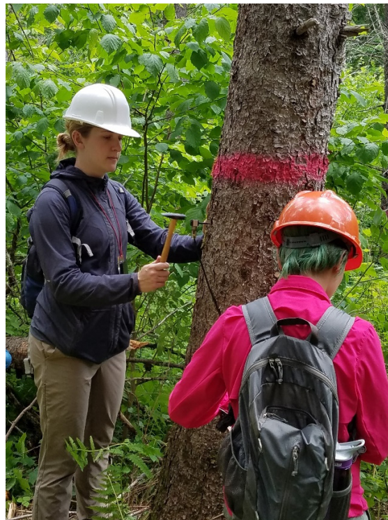
Figure 3. Transverse acoustic velocity measurements on white spruce trees using the Fakopp Microsecond Timer.
