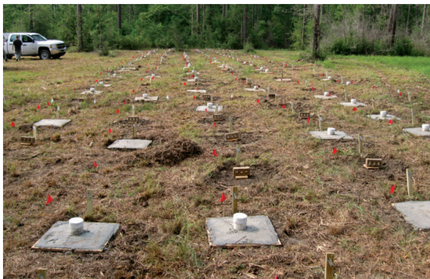
Figure 1. Completed ground board (bare soil with board and brick) and concrete slab (slab with PVC pipe) test at the Harrison Experimental Forest. Cement slab plots with no PVC pipe are soil sampling plots.
