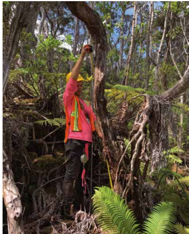
Figure 10—Field crew member Kalena Shiroma measures tree height. Tree height and diameter are used to calculate tree volume, biomass, and carbon.
