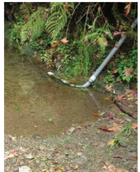
Gages such as this one in Beaver Creek, within the Smith River drainage, were positioned to measure temperature and river discharge. USDA Forest Service photo.
