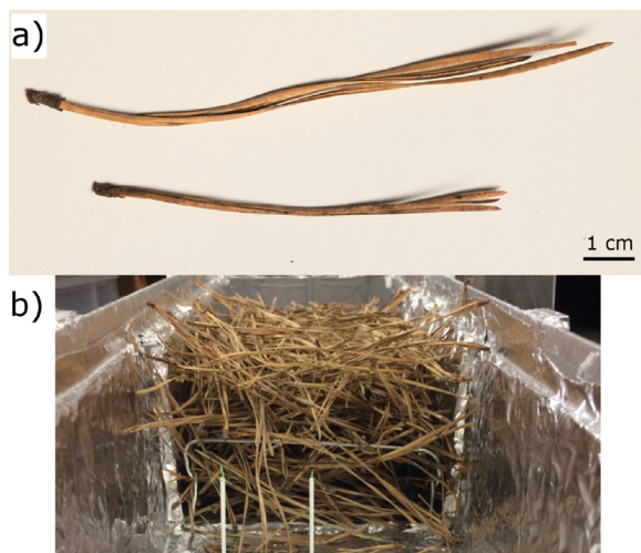
Fig. 4. (a) Example of Pinus rigida needles, which are grouped with three individual needles on one fascicle. (b) Example of fuel bed packing before test section lid is placed.
