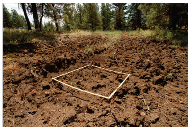
Figure 2—A sampling plot. Operating equipment under suboptimal moisture conditions can result in soil disturbance.
