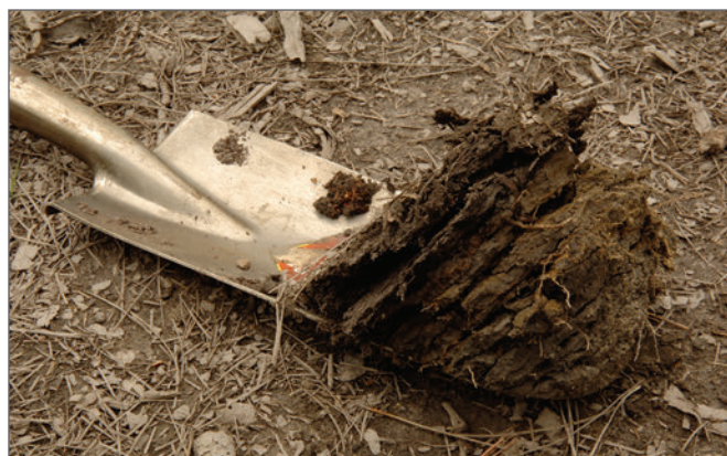
Figure 16—Platy soil structure formed on the main skid trail. Notice there are few roots within the soil.
