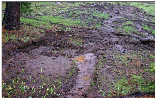
Figure 15—Puddling alters soil structure because soils are at the liquid limit and have a liquid response to external forces.
