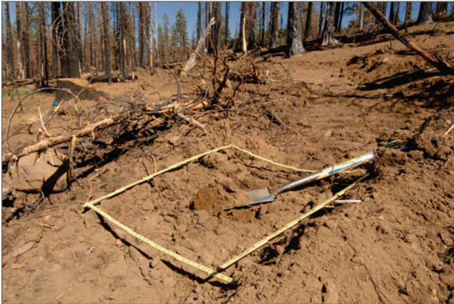
Figure 17—Platy soil structure formed on the main skid trail. Notice there are few roots within the soil.
