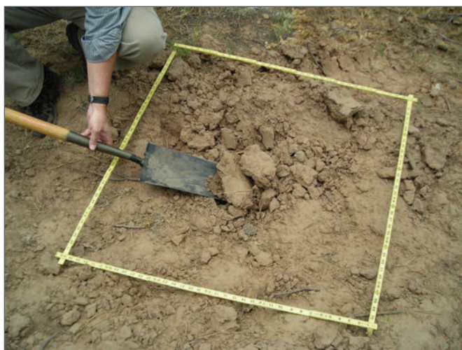
Figure 14—Soil puddling is the destruction of soil aggregates into ultimate soil particles.
