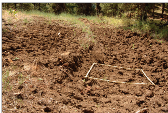
Figure 5—Rutting increases as machine traffic increases, often from repeated passes along the same route, and becomes particularly pronounced when the soil is soft due to high moisture content.
