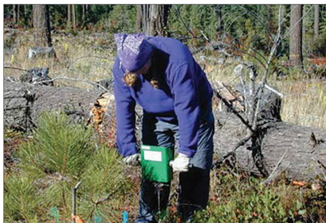
Figure 23—Typical cone penetrometer for field characterization of soil strength.
