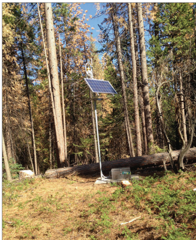
Figure 22—A remote soil sensing station installed on an off-highway/all-terrain vehicle trail system (Tahoe National Forest).
