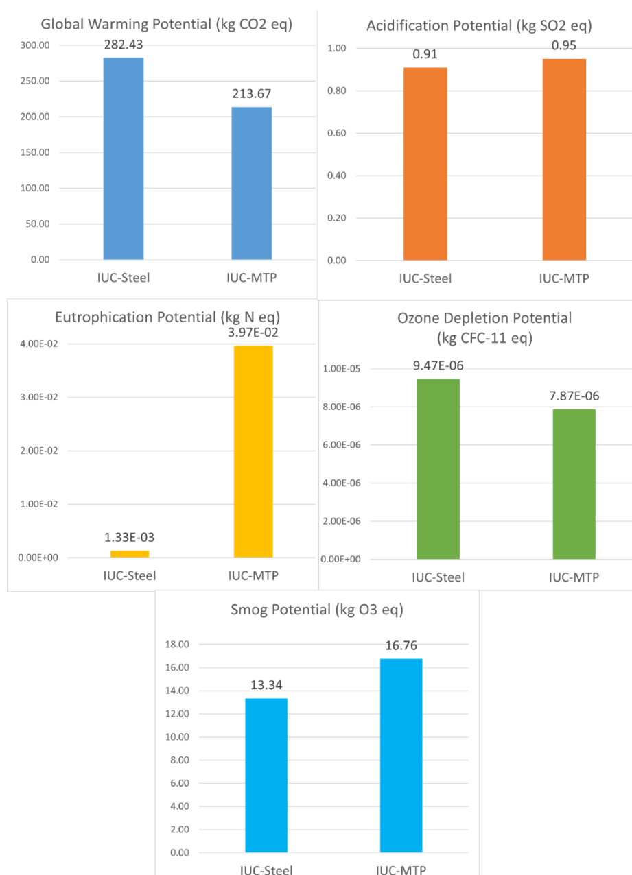
Figure 3 TRACI method reported life cycle environmental impacts from the materials used in the two functional equivalent buildings from stages A1~A3.
