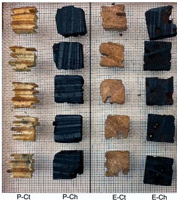
Figure 6. Test specimens post termite resistance tests (P-Ct: P. taeda control; P-Ch: P. taeda charred; E-Ct: E. bosistoana control; E-Ch: E. bosistoana charred).
