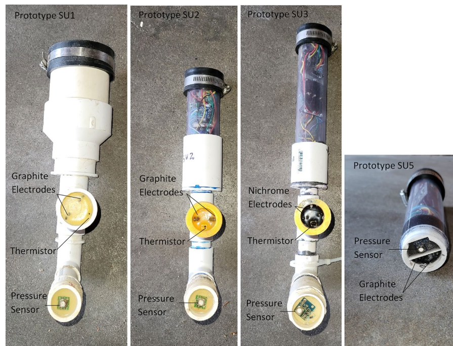
Fig. 2 Photograph of each prototype sensor. Note that the color of the potting epoxy used to waterproof the electrodes varies
