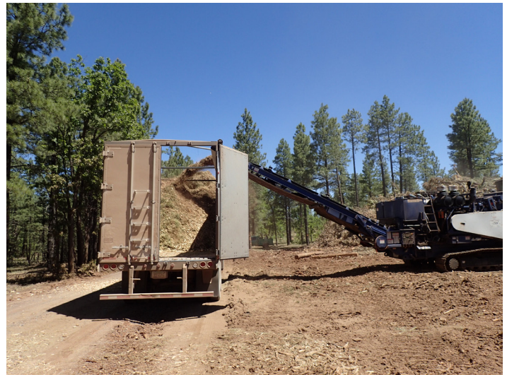
Grinder shredding biomass and loading it onto a truck for delivery to a biomass power plant. USDA photo by Nate Anderson.
