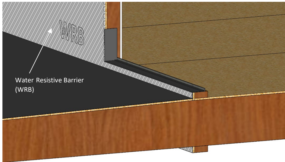
Figure 7. Install Water-Resistive Barrier (WRB)
