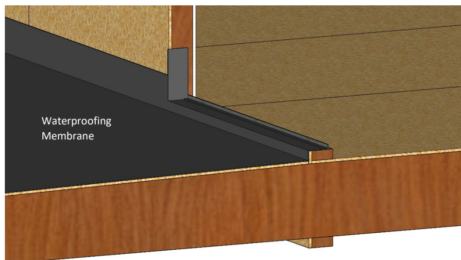
Figure 6. Install Waterproofing Membrane
