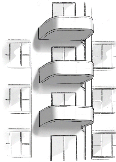
Figure 41. Dedicated Floor Drainage for Each Balcony
