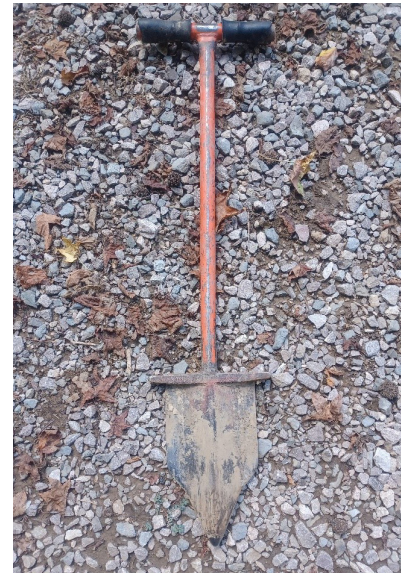
Figure 5: RA KBC bar modified to increase width of the planting bar to facilitate planting larger size seedlings. Photo Courtesy: Stacy Clark, USDA Forest Service.
