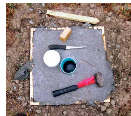
▲ Fig. 1. Treatment and concrete were completed for this plot on the previous day. The file knife will be used to remove the vapor barrier from within the PVC tube and the wood block placed inside. Finally, the cap will be placed on the tube and the identification stake hammered in the ground just above the concrete frame.
