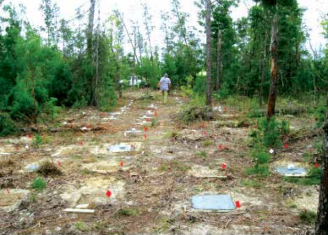
▲ Fig. 2. Completed ground board (bare soil with board and brick) and concrete slab (slab with PVC pipe) test at the Chipola Experimental Forest in March 2023. Plots with no PVC pipe or wooden boards are soil sampling plots.
