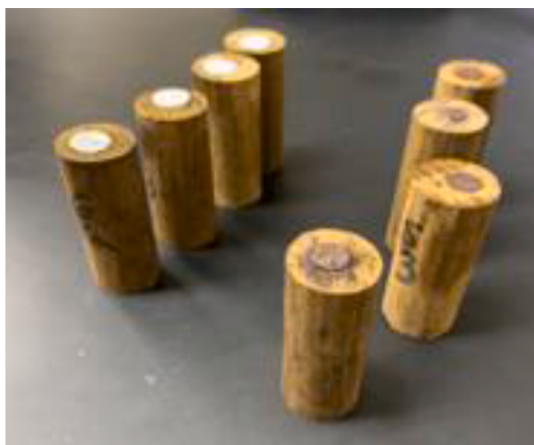
Fig. 1. Galvanized steel (left) and carbon steel (right) fasteners in the treated wood dowels tested in the isothermal calorimeter.
