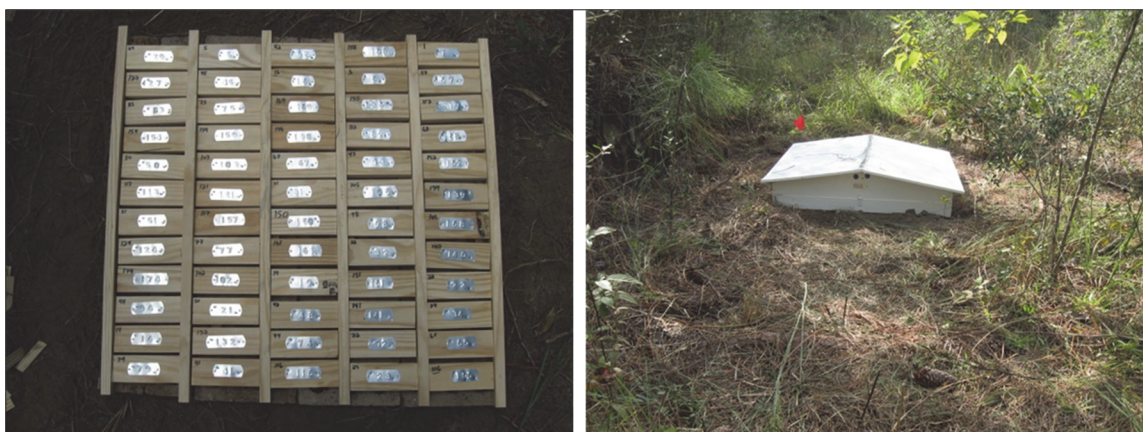
Figure 1. AWPA E26-21 Ground proximity termite test showing uncovered sample array (left) and covered array (right).
