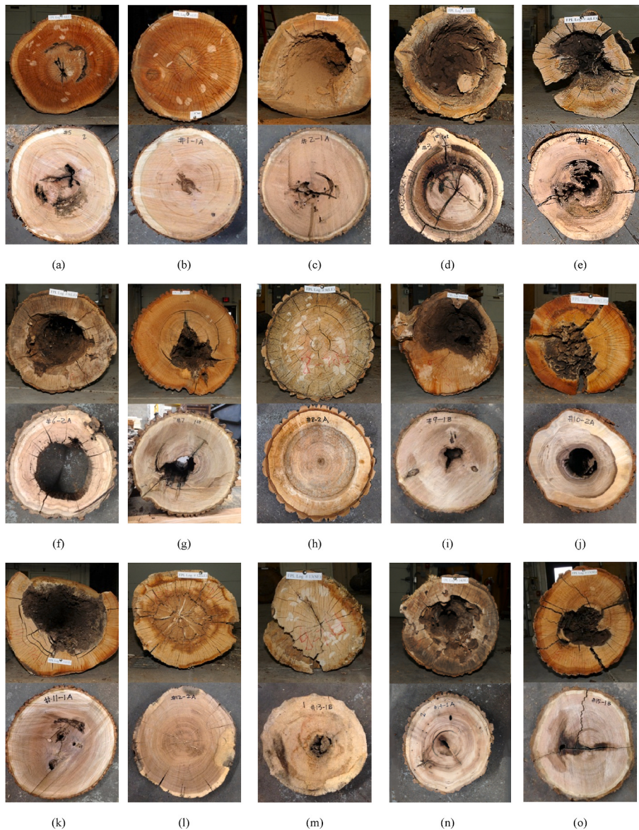
Fig. 6. Defects located in the end face and dissected cross-section of 15 logs. (a) End checks in the log no.1. (b) Rot, void, crack, etc. in the log no.2. (c) Void, crack, decay, ring shake, etc. in the log no.3. (d) Void, decay and crack in the log no.4. (e) Crack, void and decay in the log no.5. (f) Void and decay in the log no.6. (g) Void, decay and ring shake in the log no.7. (h) Ring shake and decay in the log no.8. (i) Void and decay in the log no.9. (j) Void, decay and split in the log no.10. (k) Void and crack in the log no.11. (l) Extensive check, rot, decay and end crack in the log no.12. (m) Split, surfaces decay and heart-wood decay in the log no.13. (n) Void, decay, ring shake and radial crack in the log no.14. (o) Split, internal crack (broken pieces), end crack, void and decay in the log no.15.
