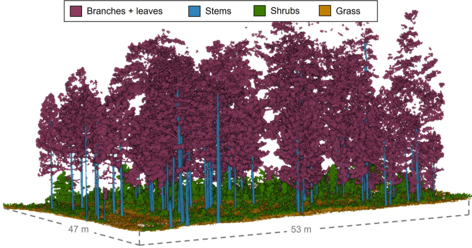
Figure 2. Terrestrial laser scanning point cloud from of a longleaf pine forest plot. Colors correspond to different vegetation structure categories that were manually classified.
