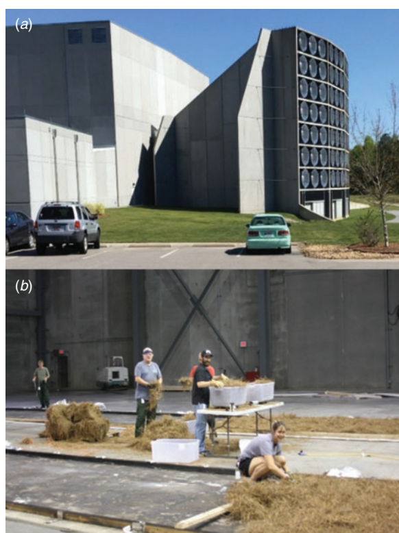
Fig. 1. (a) Exterior photo of fan array at the Insurance Institute for Business & Home Safety facility and (b) experimental chamber where staff are constructing fuel beds in preparation for a burn.
