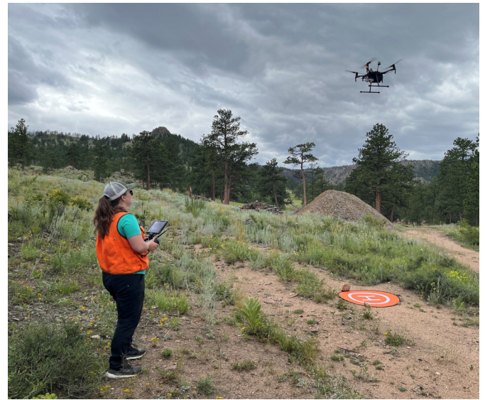
Colorado State University Ph.D. student Lauren Lad launches the UAS for its pre-programmed monitoring flight mission. USDA Forest Service photo by Wade Tinkham.
