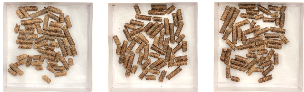
Figure 1. Fuel pellet samples of shrub willow pellets and pellets with additional lignin. From left to right: Control Pellets, RecL-Pellets, and ComL-Pellets. These samples were utilized for the measurement of pellet length.
