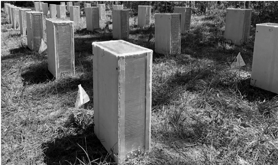
Figure 4. Field installation of CLT specimens in an RCB design ( 3 \times 10 rectangular array with 1200 mm spacing between specimens and rows) at the test site in Saucier, MS.
